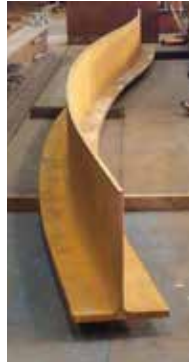
one of the beams cut into a T shape and bent at the Stelgence ® manufacturing centre to fit into the bridge
