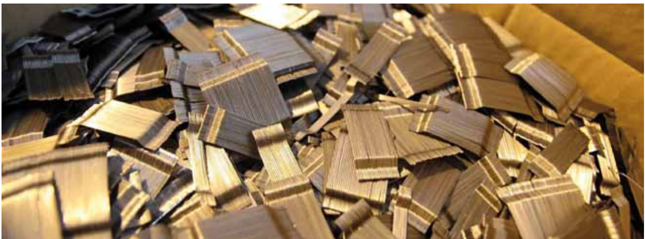
ArcelorMittal Bissen: steel fibres to reinforce concrete
